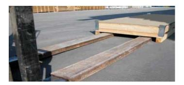
If the pallet is picked up by the short side, as may happen when unloading containers, it is necessary to use blades with a minimum length of 2.5m.
