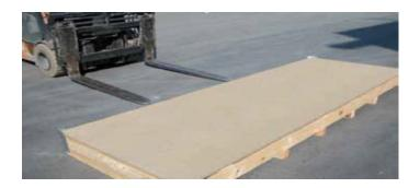
When lifting and moving bundles of 1000x3000 mm tiles with a fork-lift truck or crane, it is important to pick up the package in the centre of the long side, fully extending the forks which must support the full depth of the pallet.
